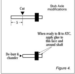
Please note that the distance between the outside ends of the Atheam bushes is about 82 mm ... the same distance as when fitted to the original Atheam motor assembly. The finished assembly will connect to the remainder of the existing cardan shaft arrangement without further modification.
